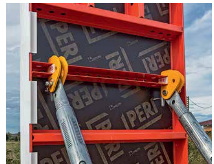
The simply designed Brace Connector can be mounted to vertical LIWA panels. For aligning horizontally-positioned panels, e.g. with foundations, the Brace Connector-2 is used.
